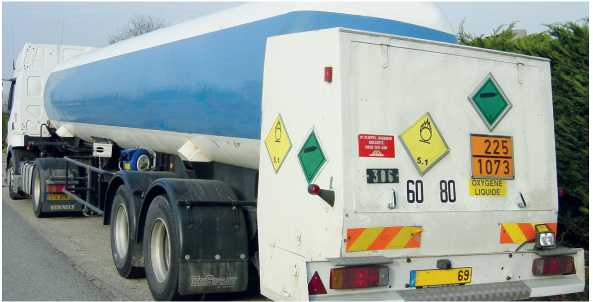
Figure 1: Example of signage for a vehicle carrying dangerous goods: green label (gas), yellow label (oxidising solid or liquid), orange plate (UN number for liquid oxygen)
