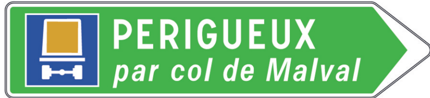
Figure 3: Example of a sign with an SC12 symbol on a diversion route
