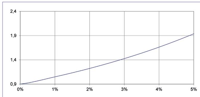
Figure 5: Change in fire rate according to tunnel gradient
