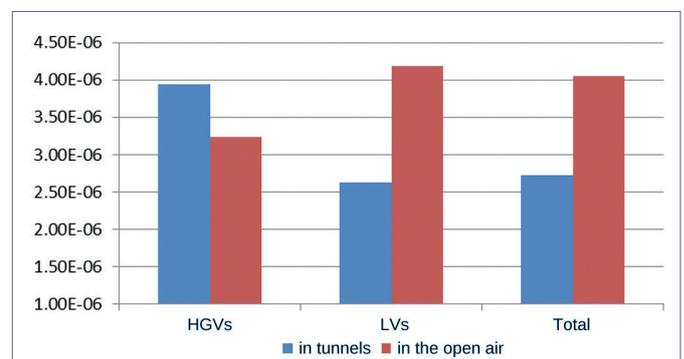
Figure 2: Average breakdown rates in tunnels and in the open air (motorways), 2008-2011
