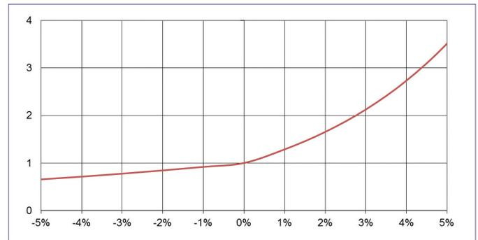
Figure 1: Change in breakdown rate according to tunnel gradient
