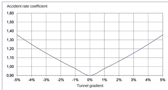
Figure 3: Change in accident rate according to tunnel gradient
