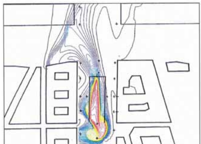
Illustration 14 - Presentation of 3D digital simulation results - Concentration curves (INERIS document)
