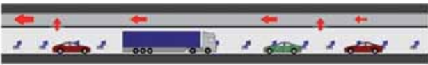
Illustration 7 - Transverse system (the arrows show the movement of air, fresh air in blue, polluted air in red)
