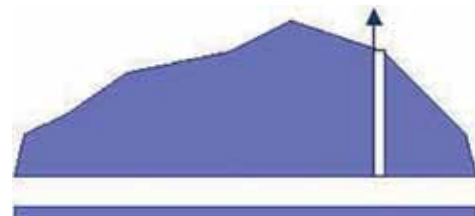
Illustration 3 - Discharge of pollution through a ventilation stack
