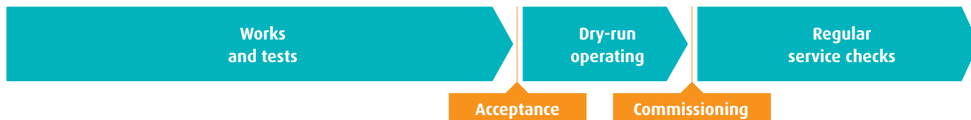
Figure 4: Simplified standard sequence for the scenario with dry-run operation positioned after acceptance of the work.
