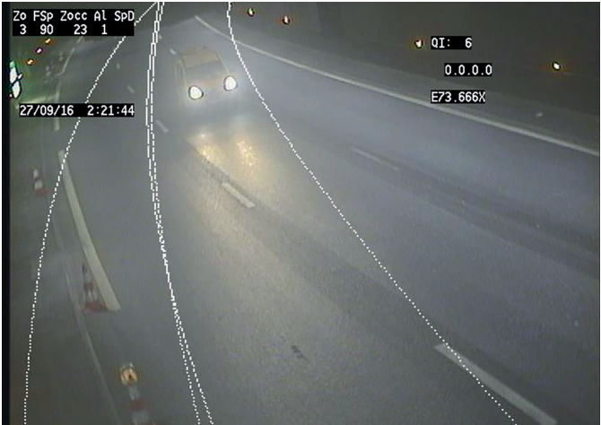
Figure 17: Video feed from a camera that has moved (misalignment of the masks)
