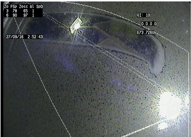
Figure 16: Poor image quality from a camera with a dirty housing window
