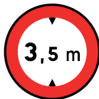
Figure 11: Type B12 sign indicating the authorised clearance gauge
