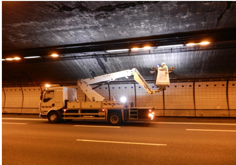
Figure 18a: : aerial basket truck of the CETU (type 2B MEWP) fitted with floodlights
