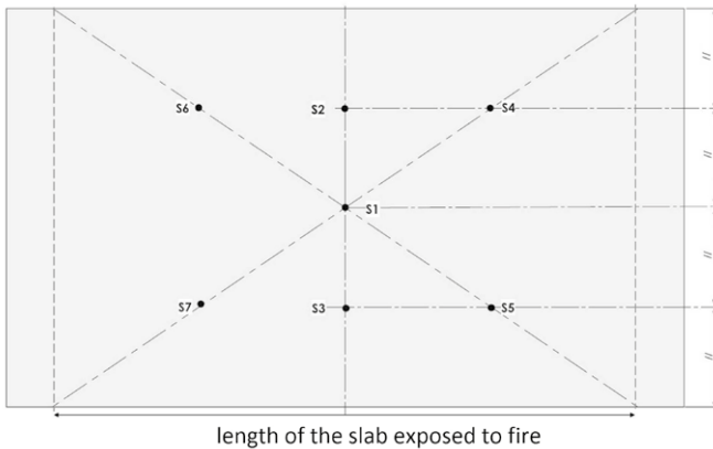
Figure A.1: positions of the sets of thermocouples in the concrete test slab (plan view)
