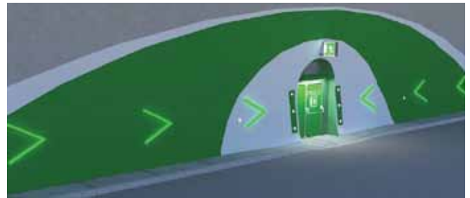
Figure 8: Example of the layout of an emergency exit with flashing lights and chevrons.
