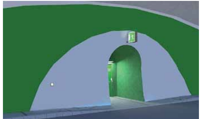
Figure 4: Example of layout of an emergency exit in recess for a D1 / D2 tunnel.
