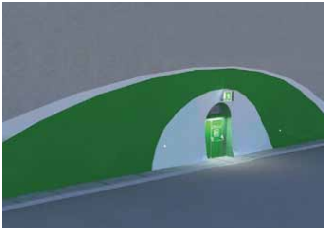
Figure 3: Example of layout of an emergency exit in a D1 / D2 tunnel.
