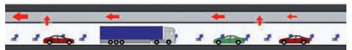
Illustration 16: transversal system - the arrows represent the direction of airflow with fresh air in blue and waste air in red (source: CETU)
